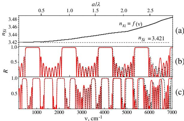
**Figure 6.** (a) Dispersion of the refractive index  $n_{Si}(\nu)$  from Ref. [14] and the reflection spectra,  $R$  calculated with (red thin line) and without (black dotted line) dispersion of  $n_{Si}$  for a 1D PC based on a Si-Air structure. The lattice constant,  $a = 4 \mu\text{m}$ , and the number of periods,  $m = 6$ . The filling fraction, (b)  $f_{Si} = 0.23$  and (c)  $0.6$  at normal incidence of light.
