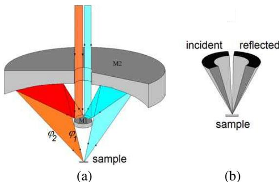
**Figure 2.** (a) Schematic of the beam path in IR microscope, showing mirrors M1 and M2 during measurements of reflection spectra  $R$ ; (b) Shape of incident and reflected light, as truncated semi-cone volumes.
