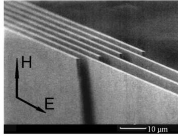
**Figure 5.** SEM image of a 1D PC with an inter-digital design. The number of periods,  $m = 6$ , and the images shows the directions of the electric field vectors, for  $E$ - and  $H$ -polarization, of the incident light.
