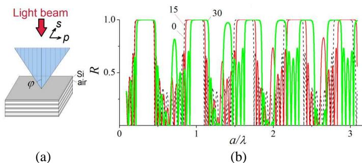
**Figure 1.** (a) Schematic diagram showing light reflection from a 1D PC (layered structure) based on “Si-Air”, with number of periods,  $m = 4$ , for calculation of reflection and transmission spectra; (b) Reflection spectra (in  $p$ -polarisation) for a specific angle of light incidence  $\varphi$ , shown by the numbers beside the curves in degrees.
