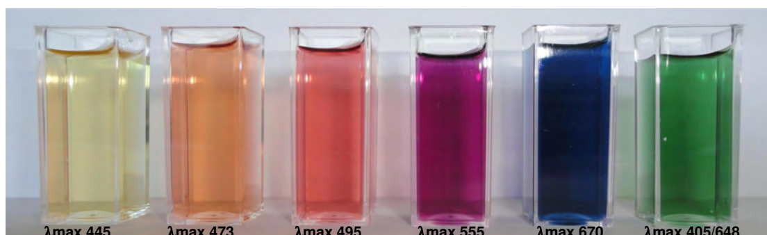
Figure 1. A sample set of the different coloured colloids produced in the practical, and their \lambda max.
