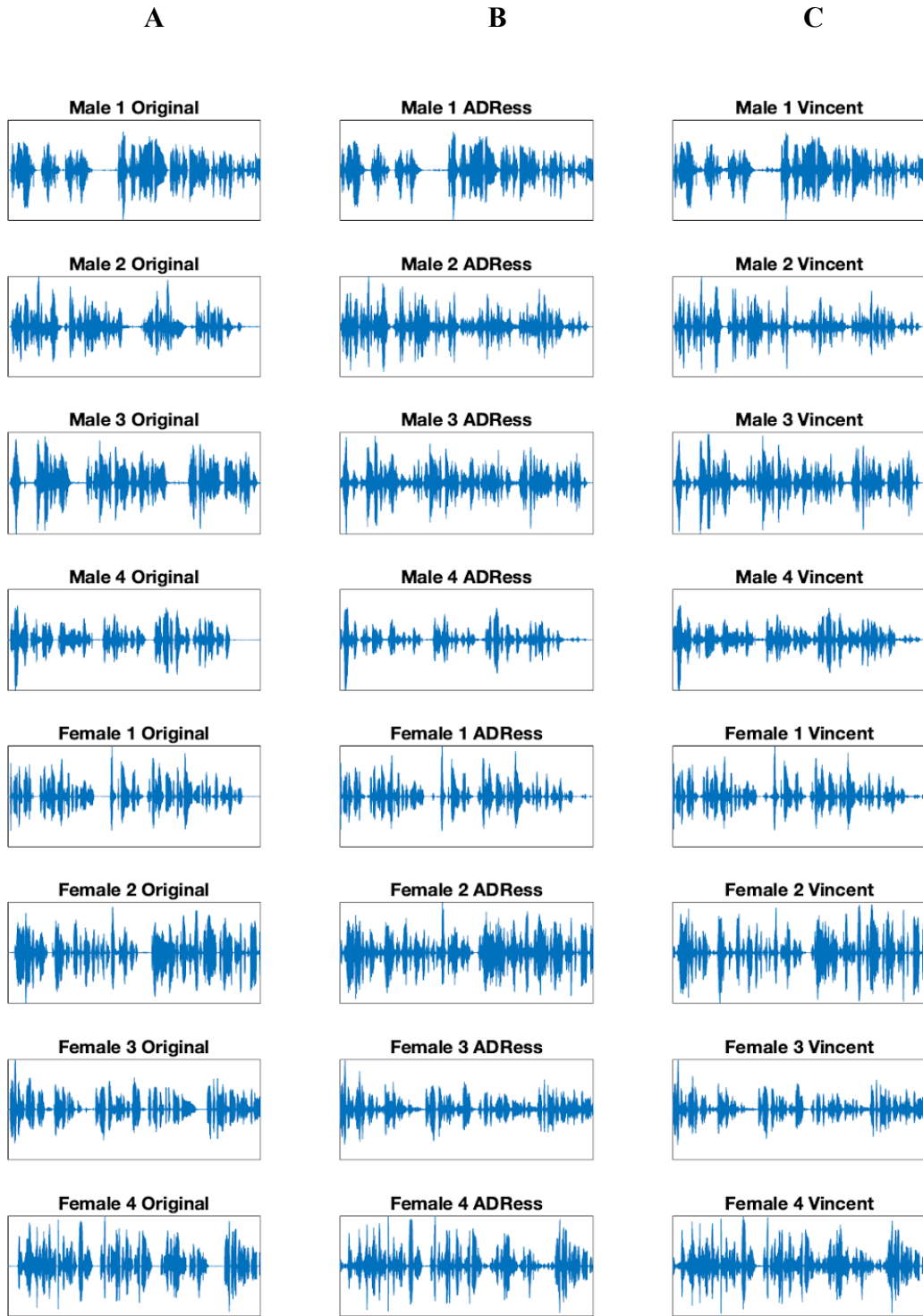
Figure 3.11 - Waveform comparisons for speech separation between A : Original sources prior to mixing, B : ADResS separations and C : (Vincent 2007) separations
