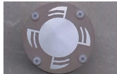
Fig. 1. Triple-band omnidirectional CP antenna (top view), as reported in [8] (under CC BY 3.0 licence).
