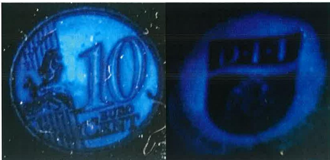
**Figure 5.13. Photograph of white light holographic reconstructions recorded with a blue laser at 473 nm.**
