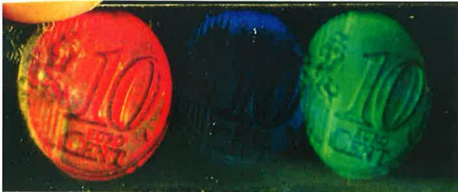
**Figure 6.23** Photograph of white light holographic reconstructions from holograms recorded at the three primary wavelengths. The object used was a 10 euro cent coin.
