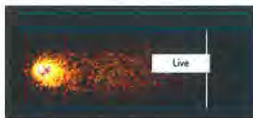
Figure 6.4 Image of a comet captured using the Komet 5.5 software and illustrating both the reading frame and the callipers used to detect and the different regions of the comet.
