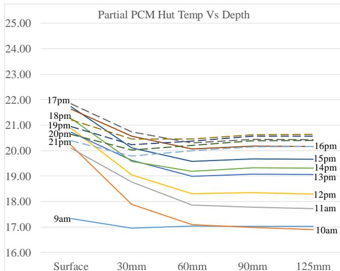
Figure 11. Temperature versus depth in the Partial PCM hut
