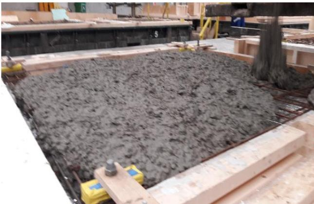
Figure 3. PCM-concrete composite panel under construction
