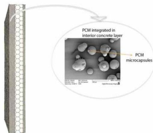
Figure 2. Precast concrete sandwich panels containing PCMs
