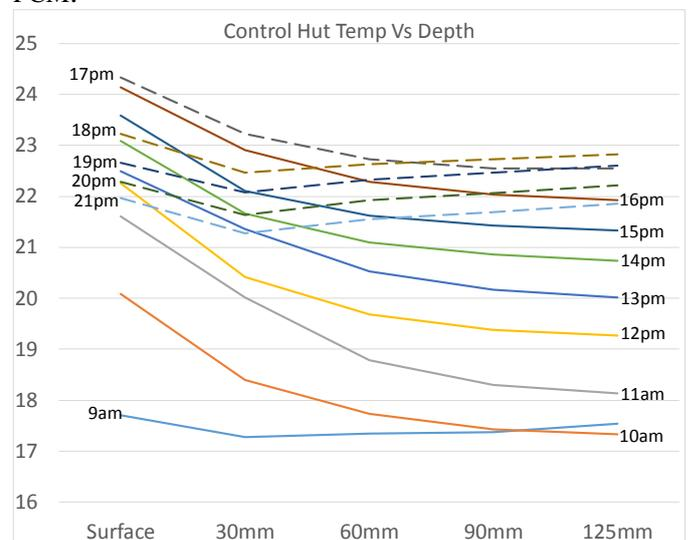
Figure 9. Temperature versus depth in Control hut
