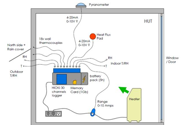
Figure 5. Schematic layout of instrumentation of each hut
