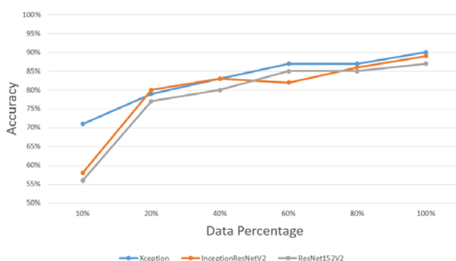
Fig. 7 Accuracies obtained with different fine-tuned models using different percentages of usage satellite dataset: Y-axis represents the accuracy of models while X-axis represents the percentage of used dataset. Blue, orange and gray lines represent the accuracy of Xception, InceptionResNetV2, and ResNet152V2 models
