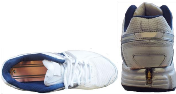
Fig. 2. Antenna inserted without insole cover.
