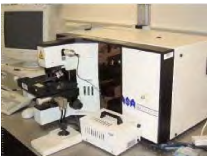
FIGURE 4.2: Instruments S.A. (Jobin Yvon) Labram 1B Raman Spectrometer
