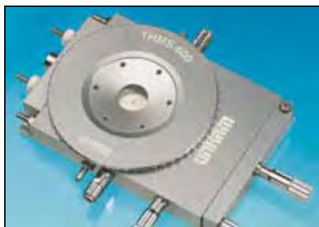
FIGURE 7.1: The Linkam Stage
