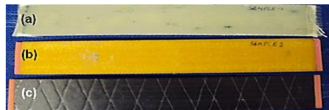
Figure 4.2 Fabricated (a) carbon-epoxy, (b) E glass-epoxy, and (c) E glass-unsaturated polyester resin composite samples
