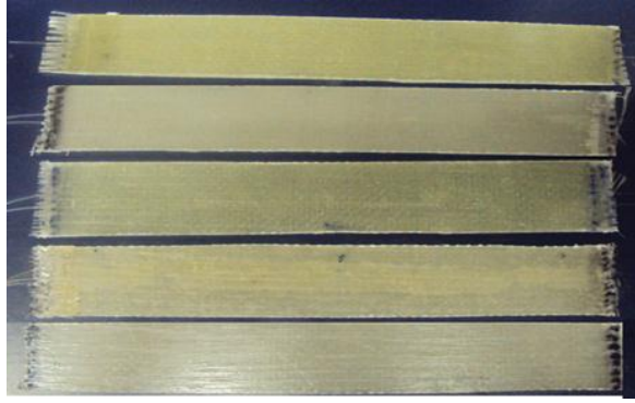
Figure A.9. Fabricated composite samples with embedded sensors.
