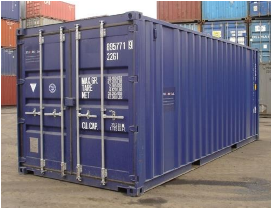
Figure 3.9: 6.06m (20' Shipping Container (TEU)
