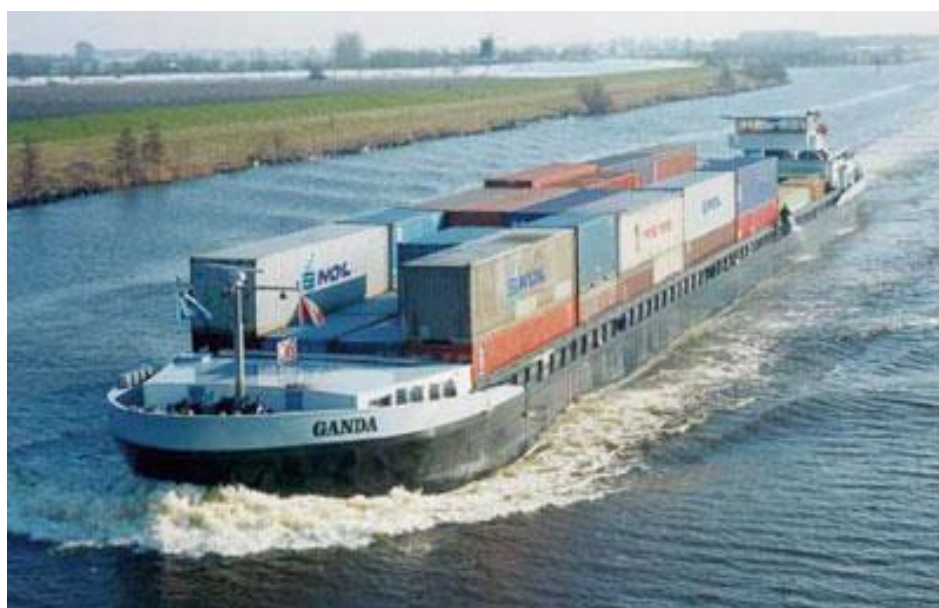
Figure 3.3: Inland canal barge with Lo-Lo containers
