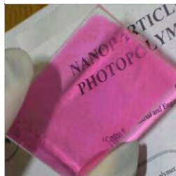
Figure 4.19. Typical layer of Beta nanocomposite film.
