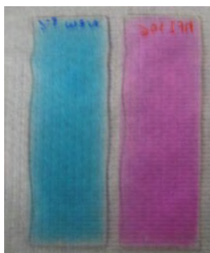
Figure 3.5. Acrylamide based photopolymer dry layers sensitized with: (left) methylene blue; (right) erythrosine B.
