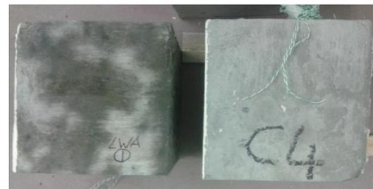
Figure 5. Leakage of PCM from the lightweight aggregate
