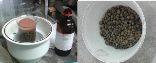
Figure 3. Manufacture of the aggregate/PCM composite
