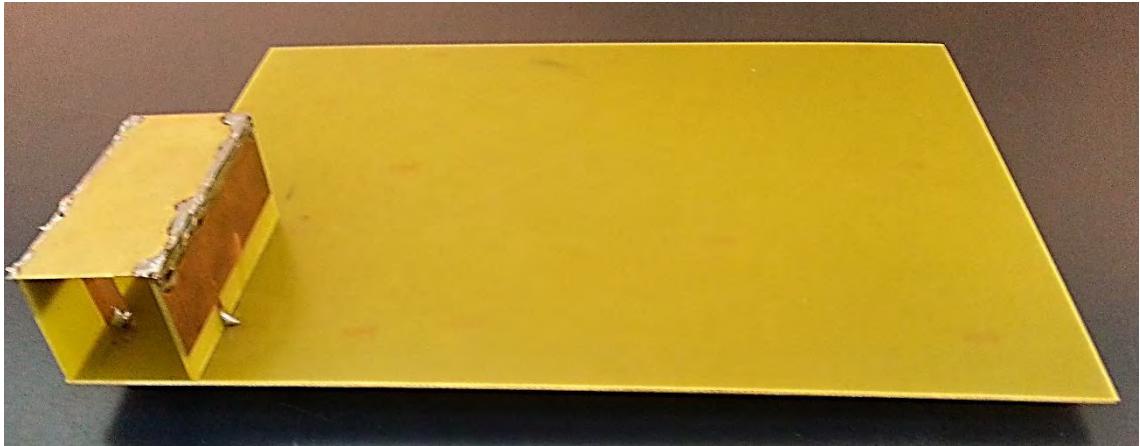
Figure 4.2. Manufactured dual band LTE PIFA prototype.
