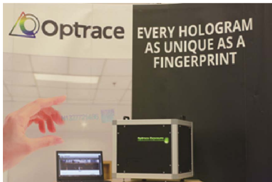
Fig. 5. Single holographic point of issue production unit. Dimensions approx. 50 cm × 50 cm × 40 cm.
