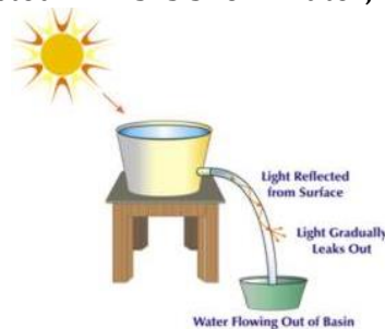
Fig. 1: Depiction of Tyndall's experiment of light reflection in a jet of water.
