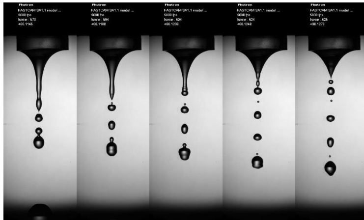
Fig. 19: Separations of the methanol satellite drop. Frames 573, 594, 604, 624, 635.
