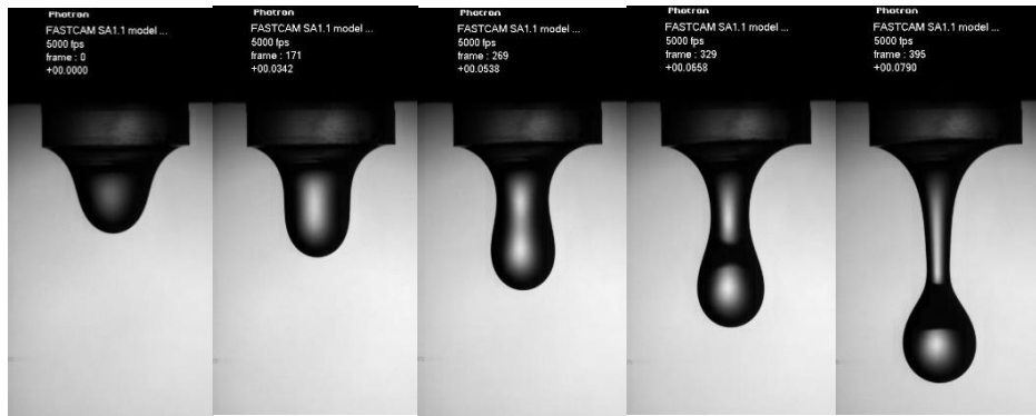
Fig. 17: Methanol drop. Frames 0, 171, 269, 329, 395.
