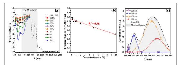
**Figure 3.** (a) Optical transmittance spectra of the various nanofluids and (b) the accompanying variation in the transmittance at  $\lambda = 385$  nm as the loading concentration of nanoparticles is increased. The spectral bandwidth over which the mc-Si PV cell operates at close to peak conversion efficiencies ('PV Window') is also highlighted in panel (a) for comparison. (c) The individual spectral components responsible for the recorded transmittance spectrum in panel (a).
