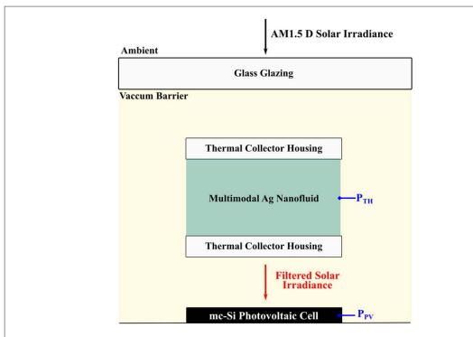
**Figure 1.** (a) Schematic of the photovoltaic-thermal (PVT) collector design formalised in the model indicating the different components in the design and the different outputs of the model i.e. the photovoltaic power  $(P_{PV})$  and the thermal power  $(P_{TH})$  produced under the optical conditions imposed by the multimodal Ag nanofluids considered in the study.
