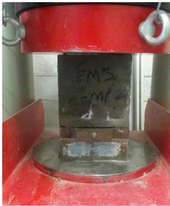
Figure 3. Cube in compression testing machine at 28 days
