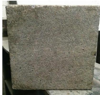
Figure 9: Surface degradation of cube from mix 1
