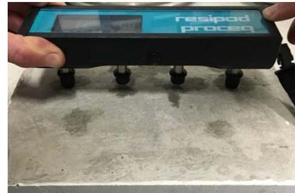
Figure 6 Resipod used for Resistivity Measurements
