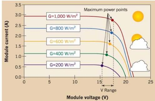
Figure 4 Typical maximum power point curve [11]
