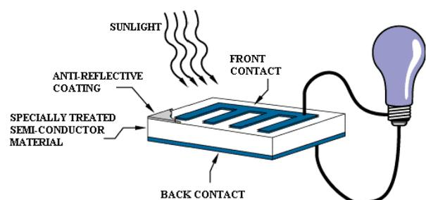
Figure 1 Operation of a Basic Photovoltaic Cell [7]
