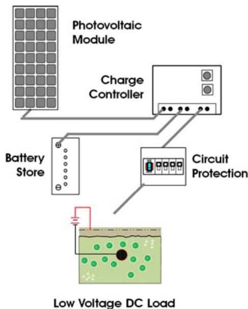
Figure 5 Block Diagram of DC PV system [12]
