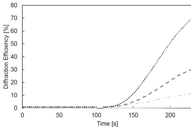
**Figure 4:** Growth in diffraction efficiency, under single beam illumination, of ‘seed’ gratings in samples prepared with different thicknesses. The grating spatial frequency is 500 lines/mm and the layer thicknesses are approximately 60  $\mu\text{m}$  (solid), 130  $\mu\text{m}$  (dot-line), 190  $\mu\text{m}$  (dashed line) and 240  $\mu\text{m}$  (dotted line). Initial diffraction efficiency is approximately 1% for the two-beam grating.
