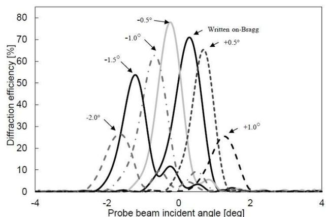
**Figure 3:** Bragg curves (the variation of diffraction efficiency with reading beam angle of incidence) for a series of gratings formed using the single beam process using different angles of incidence of the single writing beam. The layer thickness is 200  $\mu\text{m}$ . The arrows indicate the offset (in degrees) from the Bragg angle of the seed grating ( $0^\circ$ ).
