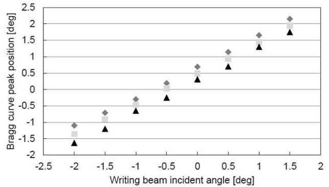
**Figure 5:** The angular position of the Bragg peak of gratings formed by the single beam process, as a function of the angle of the writing beam.  $0^\circ$  on the x axis corresponds to the angle of the beam used in writing the ‘seed’ grating. The grating spatial frequency is 500 lines/mm and the layer thicknesses are 60  $\mu\text{m}$  (diamond), 135  $\mu\text{m}$  (square), 200  $\mu\text{m}$  (triangle). Initial diffraction efficiency is approx. 1% for the two-beam grating.
