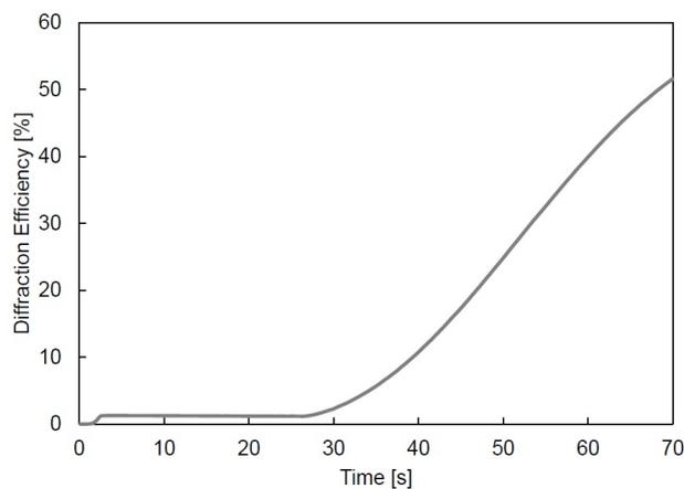
**Figure 2:** Diffraction efficiency versus exposure time. A standard two-beam holographic recording of 2 seconds is followed by a 25 second delay (no illumination) and then illumination with just one of the writing beams. Exposure intensity is 2.5  $\text{mW}/\text{cm}^2$  in each beam
