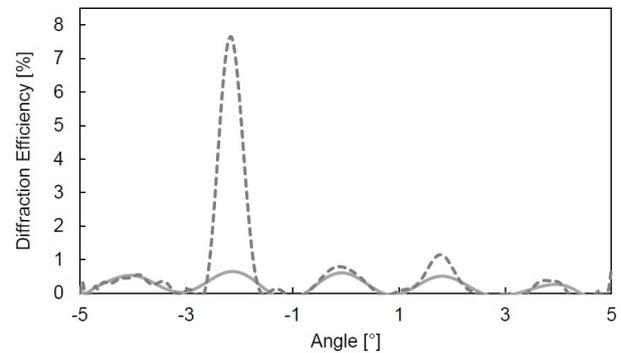
**Figure 7:** Variation of diffraction efficiency with reading beam angle of incidence for a series of gratings, from which one individual grating has been enhanced by illuminating with a single on-Bragg beam of light. The angular separation between neighbouring gratings is  $2^\circ$ .
