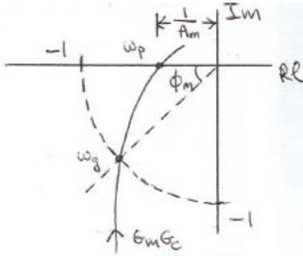
$$\text{Then } G_m(j\omega)G_c(j\omega) = \frac{K_m K_c \sqrt{1 + \omega^2 T_i^2}}{\omega T_i \sqrt{1 + \omega^2 T_m^2}}$$
