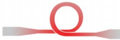
Figure 2.6: Schematic diagram of a microfiber loop resonator (taken from [70]).
