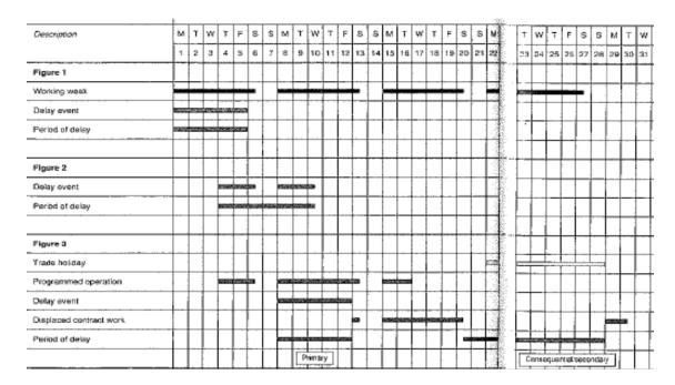
Figure 1 – Effect of Delay Events on Programme Durations (source Birkby and Brough)
