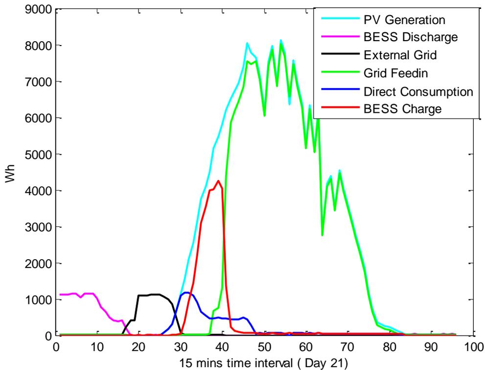
Figure 6: Energy Flow signals obtained from EM controller
