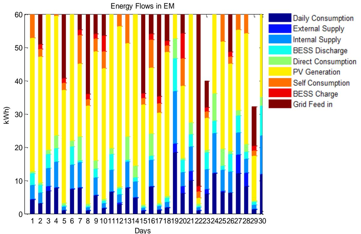
Figure 5: Energy Flow signals obtained from EM controller
