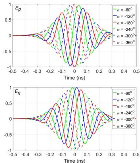
Fig. 3:  $E_p$  and  $E_q$  components of received pulses as a function of  $\alpha$
