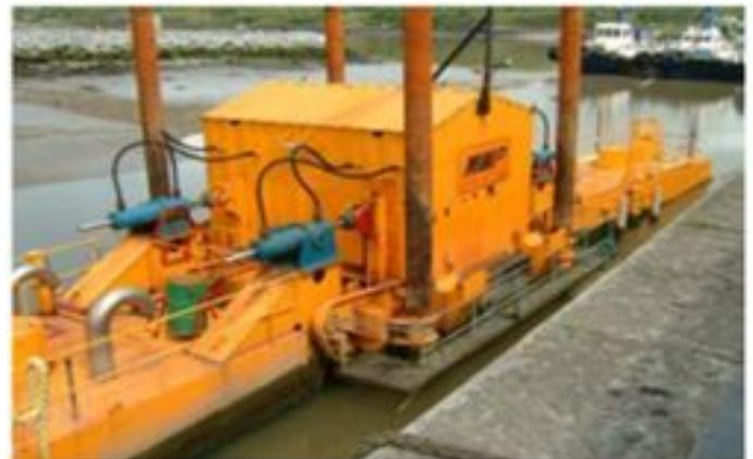
Fig. 12. McCabe Wave Pump device.
