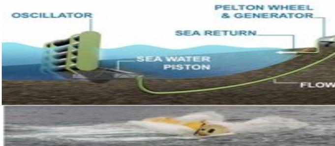
Fig. 7. The Oyster device by Aquamarine Power.
