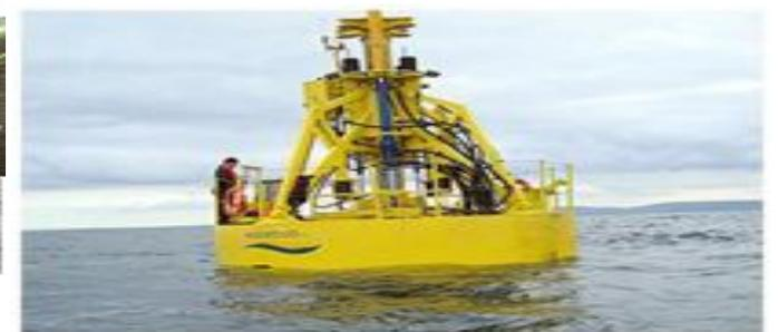
Fig. 9. The Wavebob device.
