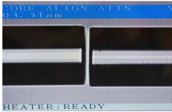
Fig. 6 Screenshot of the splicing process using attenuation splicing mode.
