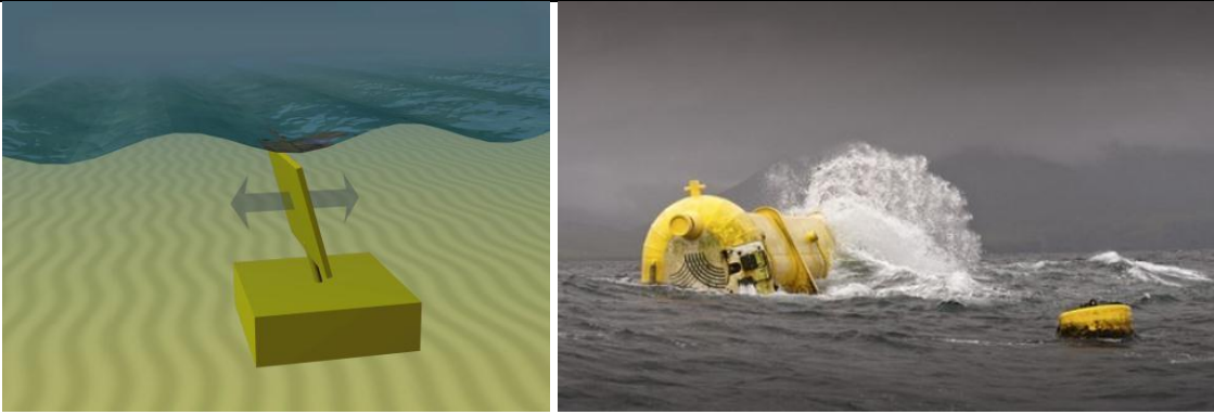
Oscillating Wave Surge Converter Operating Concept and Example (Courtesy Aquamarine Power Ltd.)
