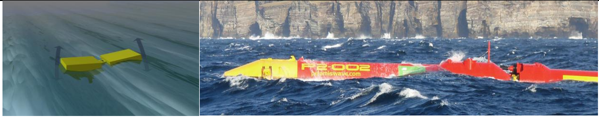
Left: Attenuator Operating Concept (Courtesy Aquaret) and Right: Example (Courtesy Pelamis Wave Power Ltd.)
