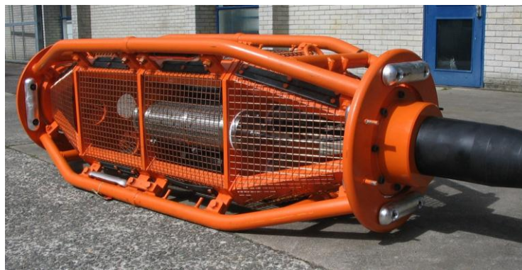
FIGURE 3.10 J&S LTD. SPLICE HOUSING (COURTESY J&S LTD)
