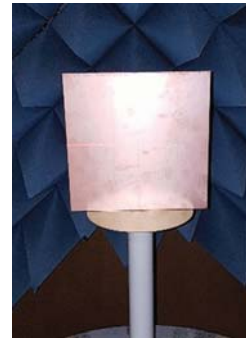
Fig. 3. Reflecting plane for system origin calibration.
