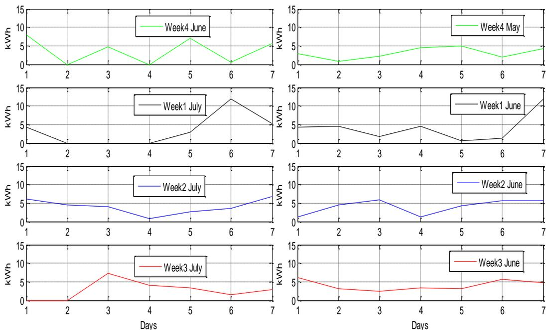
Figure 3: Sample Load profile (May-June, June-July)
