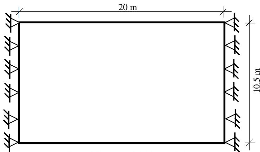
Figure 3 Plan view of slab bridge deck
