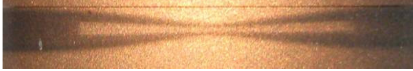
Figure 1. An image of one of the fabricated PCF tapers.
