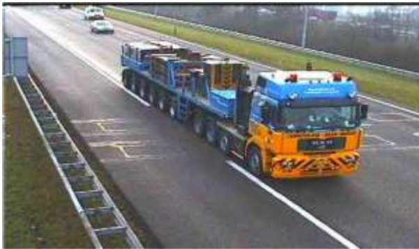
(c) Crane ballast truck (109 tonnes, 10 axles).
