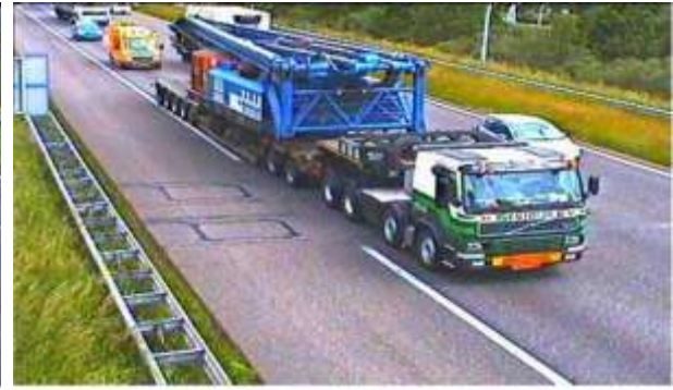
(b) Low loader (127 tonnes, 11 axles).
