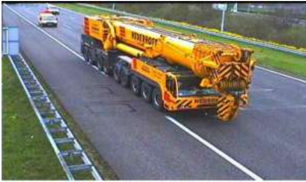
(a) Mobile crane (109 tonnes, 9 axles).
