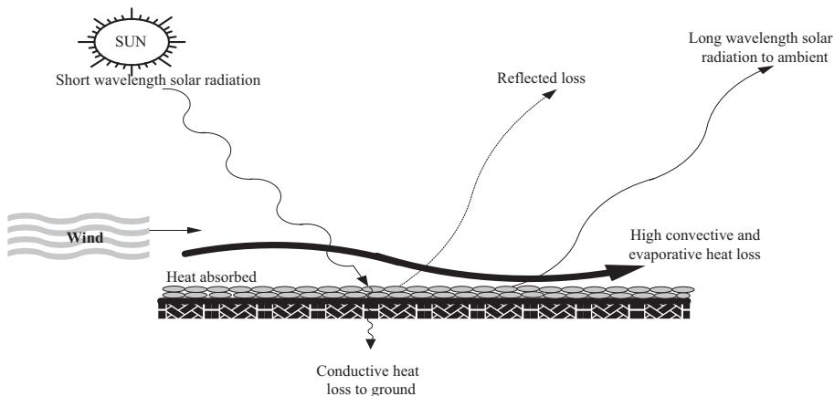
**Fig. 8.** Open sun drying.
