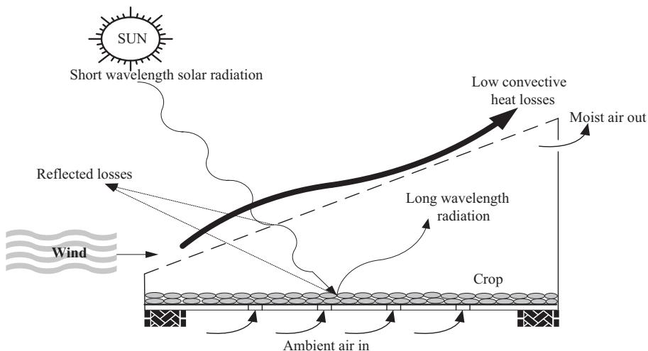
**Fig. 9.** Schematic diagram of direct solar drying.
