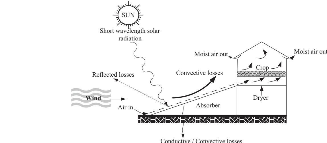
**Fig. 10.** Indirect solar drying.
