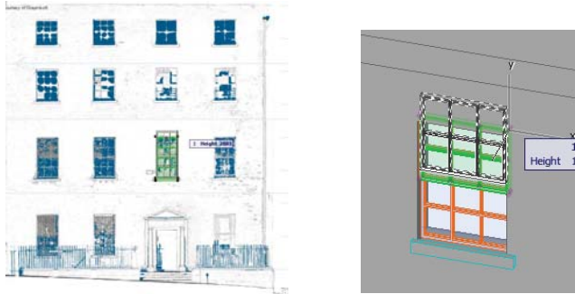
Figure 6. Interactively Modifying Position of Window Openings
