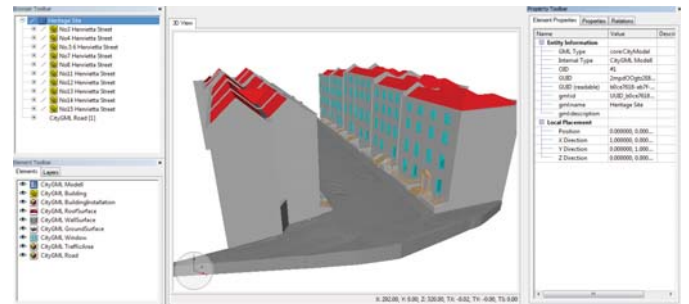
Figure 17. CityGML Model Showing Semantic Classes.
