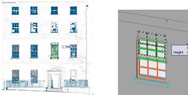
Figure 6. Interactively Modifying Position of Window Openings
