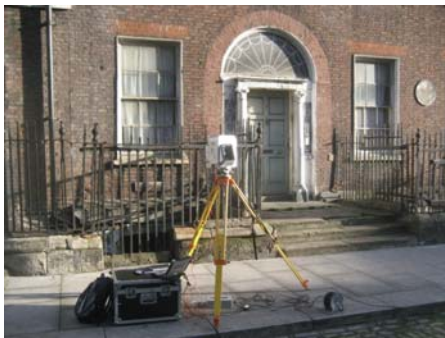
Figure 9. Trimble GS200 Laser Scanner
