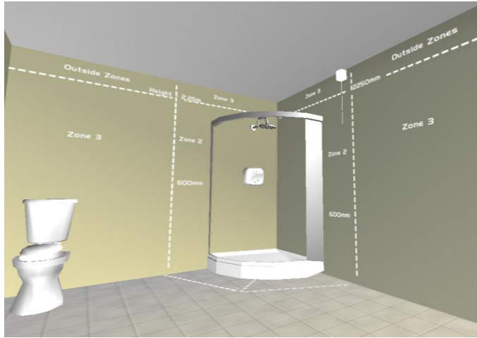
Figure 4 View of Zones in bathroom in VES
