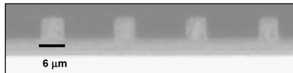
Fig. 15. Cross-sectional view of photopatterned waveguides.
