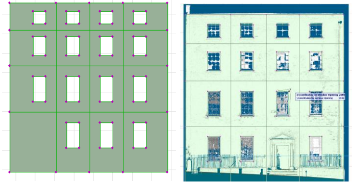
Figure 7. Wall façade with editable points marked (left) & Wall façade overlaid with survey data (right)
