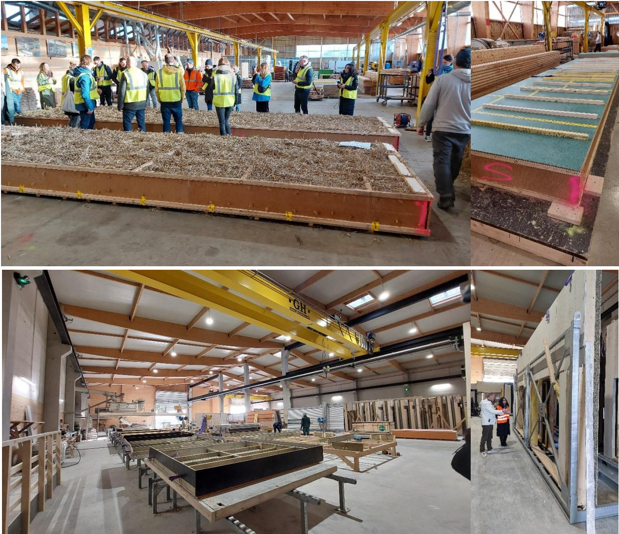
Figure 17: Showing straw based (above) and hemp based (below) biobased modular wall panel manufacturing facilities. Chênelet (straw) & Wall'Up Prefa (hemp) Northern France [Source Authors].
