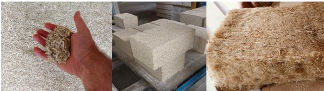
Figure 16: Showing range of hemp based resource materials and products (shiv, hempblocks, and hemp fibre batts). Senini-Tecno Canapa Northern Italy [Source Authors].
