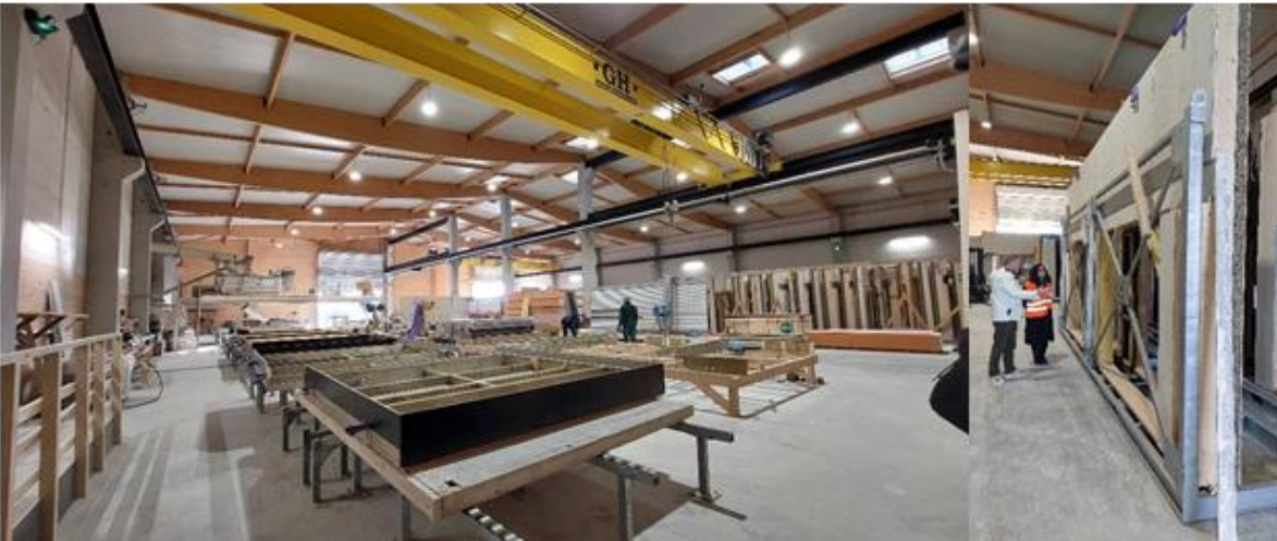
Figure 12: Showing hemp lime modular wall panel manufacturing facility, showing factory floor assembly and storage areas LHS and large complete wall panel with lifting / support frame, RHS. Wall'Up Prefa northern France [Source Author].
