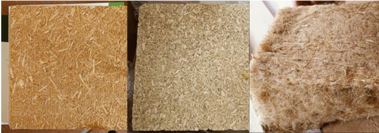
Figure 10: Showing examples of boards, batts and quilts from biobased agri-crops straw, hemp, miscanthus. LHS Straw board from VestaEco northern Poland, Centre Miscanthus board from Miscanthus-Buscheritz east Germany and RHS Hemp batt from Senini-Tecno Canapa northern Italy [Source Author].
