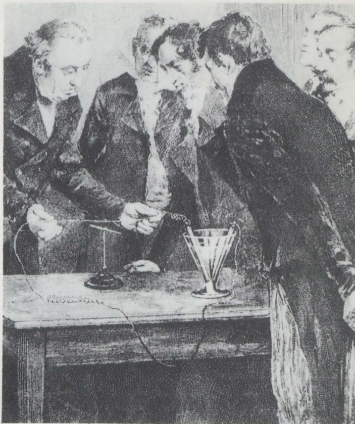
OERSTED, Professor at the University of Copenhagen demonstrating to his audience the effect of electric current on a pivoted magnetised needle.
