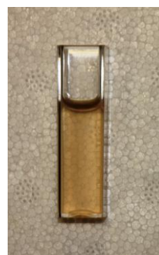
Fig.3: QD 570 dispersed in epoxy resin and casted in 1cm polymethylmethacrylate (PMMA) cuvette.
