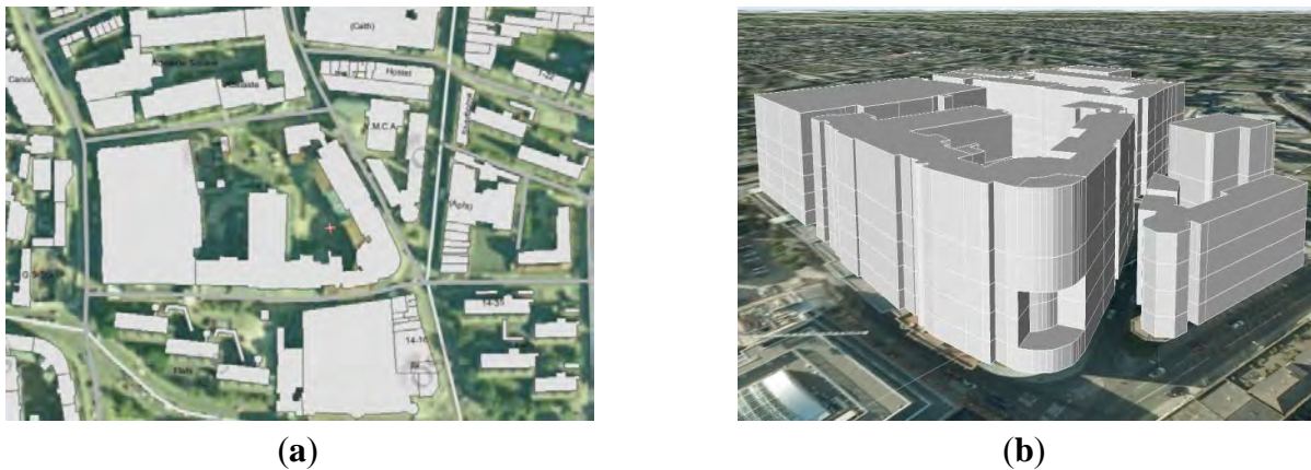
Figure 5. A true 3D (geometrically accurate) model of a campus building derived from detailed laser scanning. Individual features are stored separately in the database.
