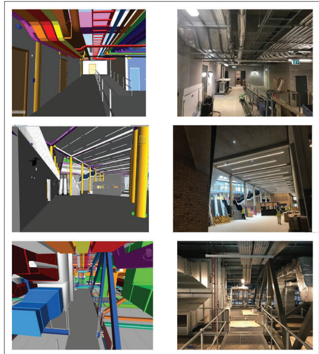
Image 2: Synchronized MEP BIM model applying MagiCAD (Case Study Project).
