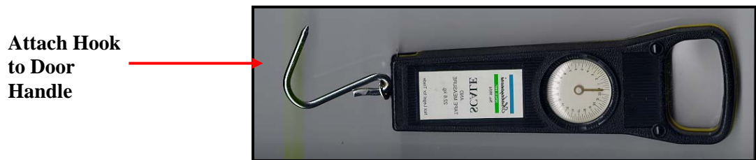
Figure 2.5 Scanned Image of Force Metre used to Measure Torque
