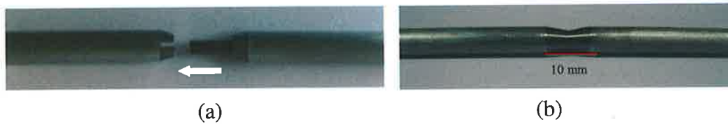
Figure 3.2 Paired metal rods (a) separate milled rods, each having 5 mm constriction (b) Coupled rods representing a 10 mm axial constriction at centre
