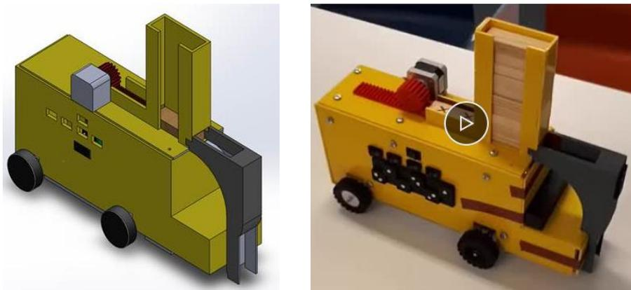
*Figure 2: An example of the interim CAD model and final block dispensing robot built by students in 2017-18*
