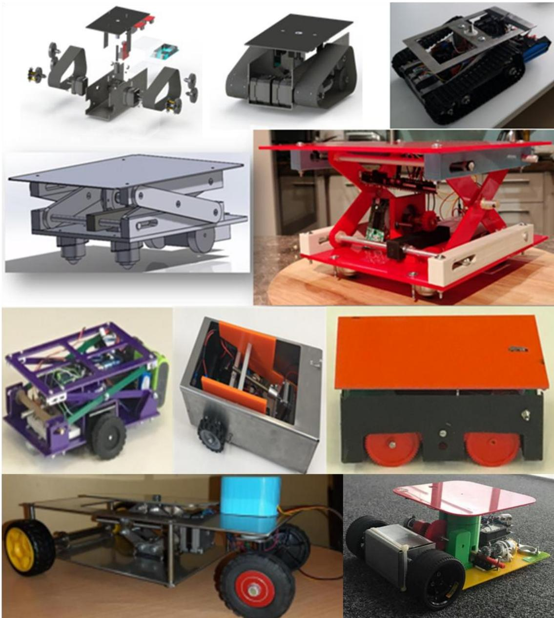
*Figure 3: Examples of CAD models and some of the semi-autonomous warehouse picker robots built by students in 2018-19*
