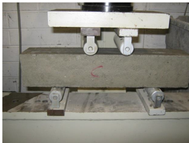
Figure 5 Test setup for the flexural test
