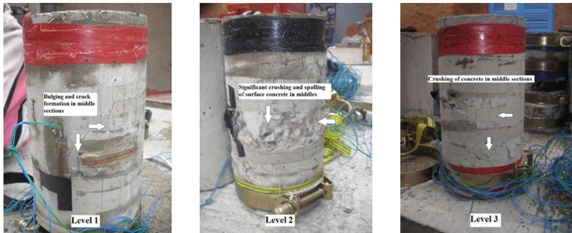
Figure 20 Test Series 4 cracked specimens.
